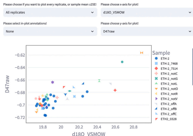
Fig. 4. Demonstrative screenshot of the Discover Results page, displaying \delta^{18}\text{O} data vs. \Delta_{47, raw} data for individual replicates of carbonate standard ETH-2. \text{CO}_2 - \text{H}_2\text{O} re-equilibration is indicated for replicates showing both elevated \Delta_{47, raw} and \delta^{18}\text{O} values. \Delta_{47, CDES90} values of these samples plot outside the long-term repeatability interval characteristic of ETH-2 ( 0.2093 \pm 0.0017 \text{ ‰} ) in the absence of significant analytical bias [36].
